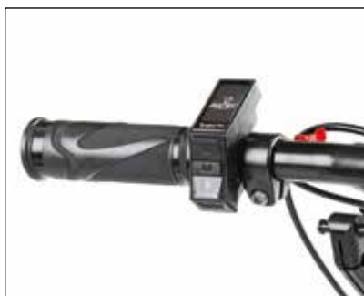
TFT colour display, LED lights and buttons.
